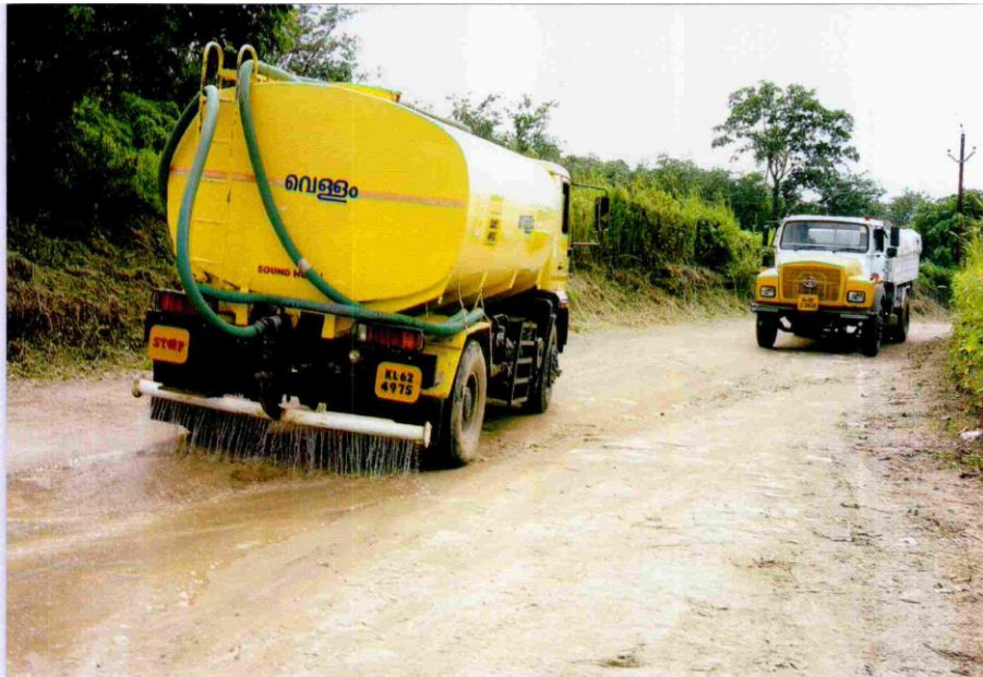
Fig 3.1 Water tanker with sprinkler
