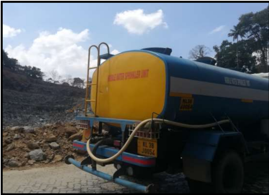
Water Tanker with sprinklers
