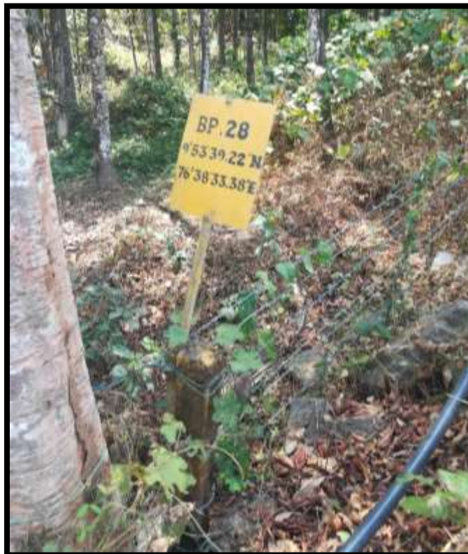
Boundary Pillars with location co-ordinates & barbed wire fencing
