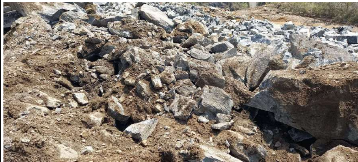
Fig 12: Fragmented Rock after Blasting
