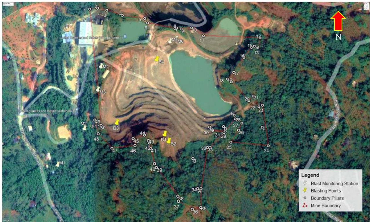
Fig 3: Google Earth Image of the Mine showing Blasting Locations & Monitoring Points
