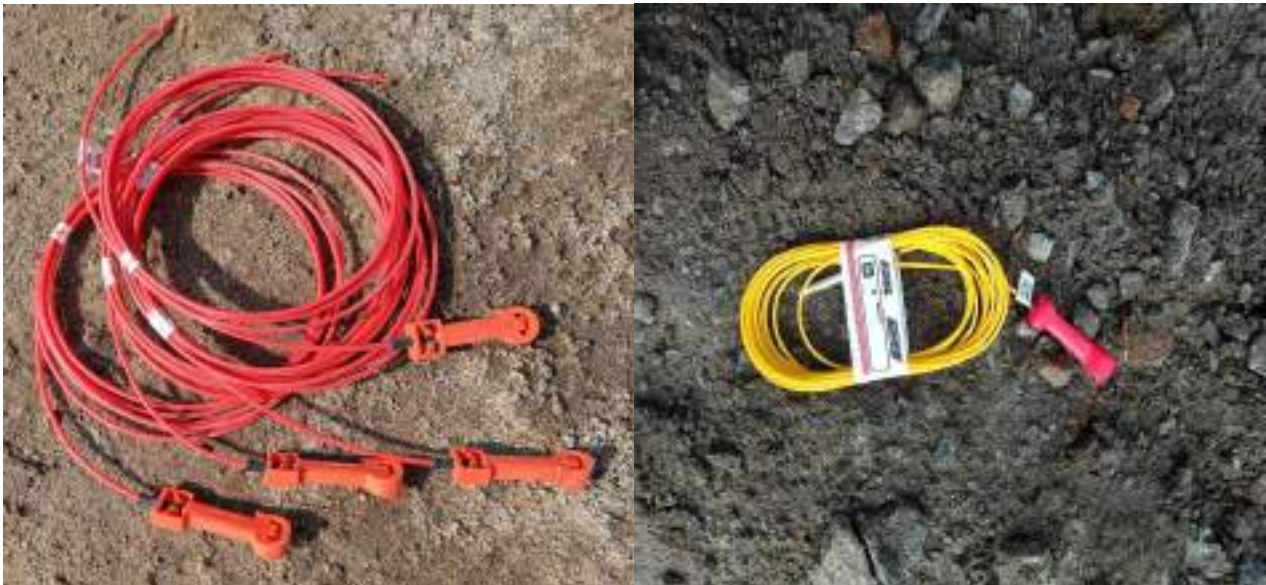
Fig 8: Non-Electric Detonator & Surface Trunk Line Delay used in the Quarry
