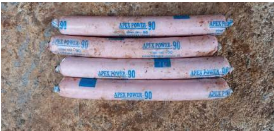
Fig 9: Explosive Cartridges used in the Quarry
