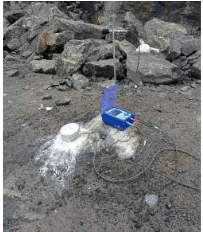
Fig 14: Blast Vibration Monitoring
