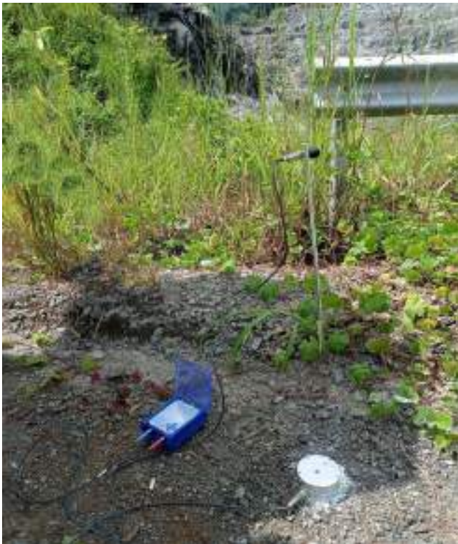
Fig 14: Blast Vibration Monitoring
