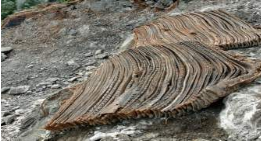
Fig 12: Muffling arrangements to control the Fly rocks
