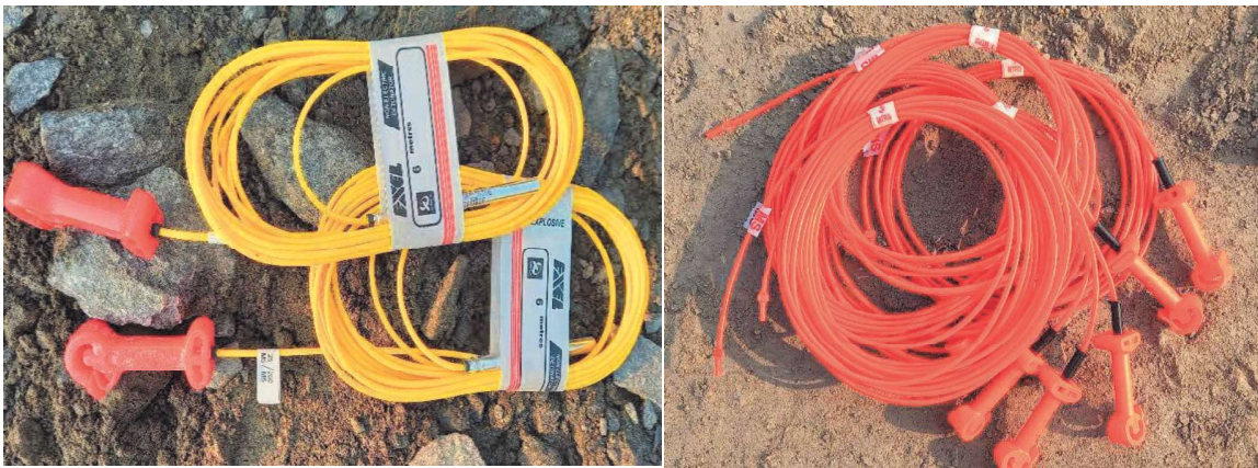
Fig 8: Non-Electric Detonator & Surface Trunk Line Delay used in the Quarry
